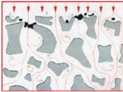
Fig. 5 – Settling of particles on the surface
