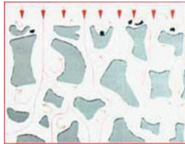
Fig. 6 – Filtration by accumulated particles
