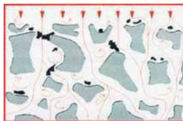
Fig. 10 - X-ray analysis shows the ability of the filter to reduce the turbulence of the metal flowing into the casting
