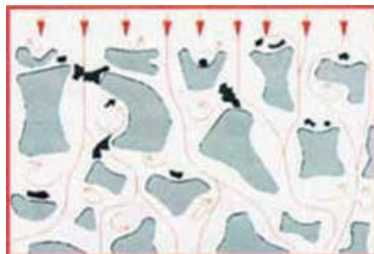
Fig. 7 - Filtering inside the filter
