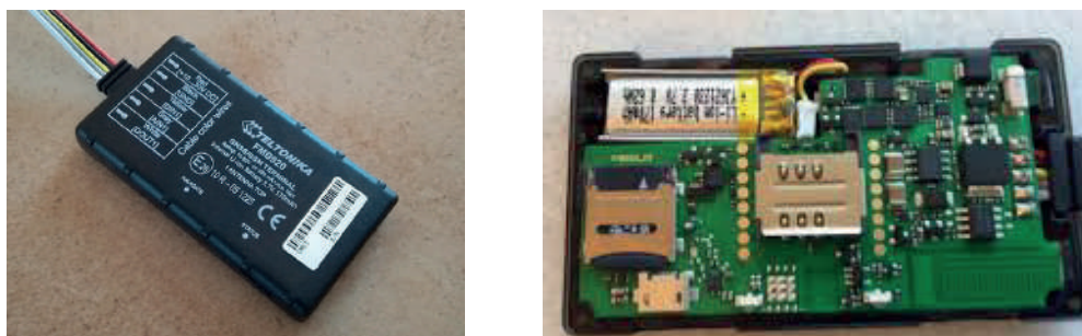
Fig. 2. GPS receiver Teltonika FMB920 installed in combine Dominator-130.
